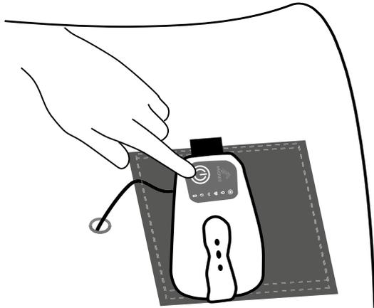
Turn the EQUIMETRE off by pressing the button during 3 secondes. All LEDs should turn off.
